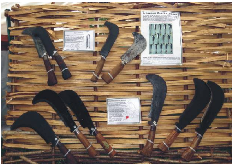
Devon billhooks are displayed in the bottom row, above are much lighter hooks used for splitting thatching spars. The main distinguishing features of Devon billhooks are a pronounced nose and a notch cut into the blade at the handle end. Blackdown Hills Hedge Association display board.
