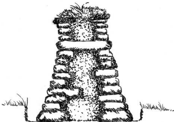
Figure 1: Banks, whether stone or turf faced, should have concave faces for strength. When stone faced, the largest stones should be at the base. Heather Harley after original in first edition
