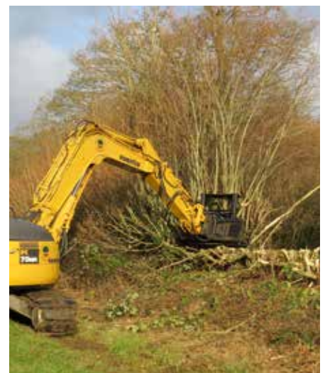
Right: Coppicing a hedge for woodfuel using a felling head with tree shears
